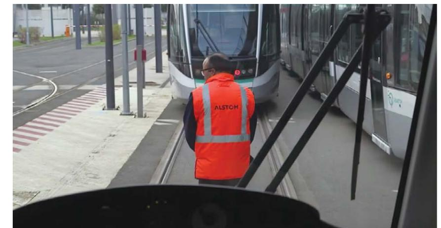
Parisian operator RATP carried out a pilot with 'driverless' tram stabling in conjunction with Alstom in 2017. A retrofitted Citadis manoeuvred itself around the T7 depot in Vitry-sur-Seine, following staff members around at safe distances and stopping at designated stabling positions. RATP/Alstom
